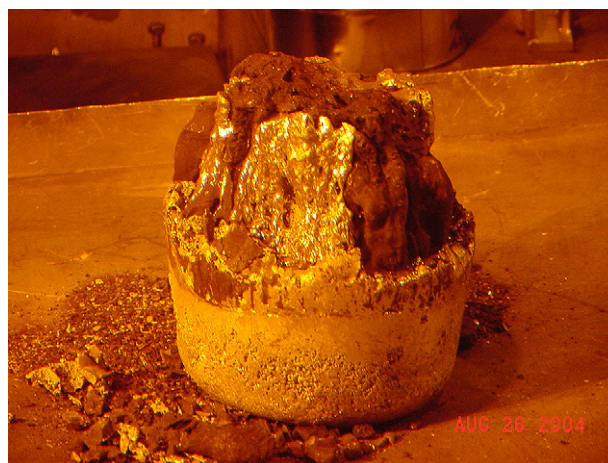
Fig. 4. Photograph of condensate ingot following cadmium distillation experiment.
