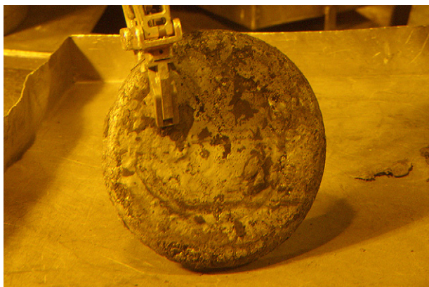
Fig. 3. Photograph of plutonium–uranium ingot following cadmium distillation experiment.
